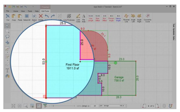
With the 53' wall selected tap 5 on your keyboard (because we need to move the line 5' to the left) and tap the left arrow on your keyboard. This will move the 53' wall 5' to the left, extending the two attached walls.
