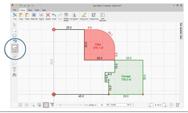
**Note**: Once you are back in Draw Area Mode with the "pen down" at one end of the open area you can hit the delete key to delete additional lines of the open area.
